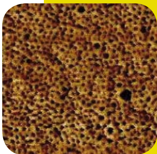
AFM image of a thin diblock copolymer film with one block as cylinders oriented perpendicular to the substrate. (a) AFM phase image, (b) model, (c) grazing-incidence small-angle x-ray peak showing that the cylinders penetrate through the whole film.
